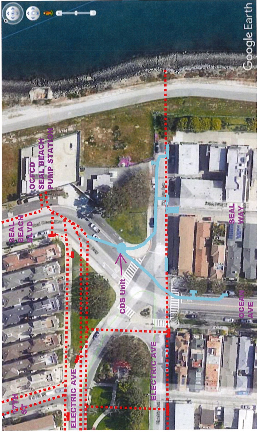
Figure 2 – Proposed Storm Drain Facility
